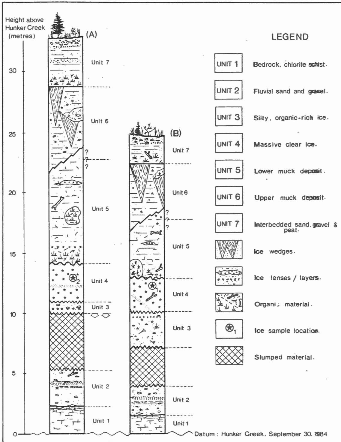
Figure 3. Two detailed stratigraphic sections illustrating relationships between ground ice bodies and enclosing sediments, Mayes Claim, Hunker Creek.
