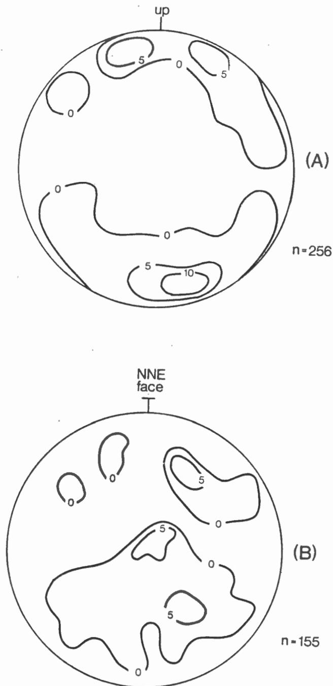
Figure 12. Fabric diagrams for ice sample #2. (A) C-axis distribution from 2 vertical thin sections for planes oriented normal to the thaw face and oblique to the local slope. The sample represents approximately 35% of the total number of crystals visible in the thin sections. (B) C-axis distribution for 155 ice crystals from 2 horizontal thin sections within the sample.
