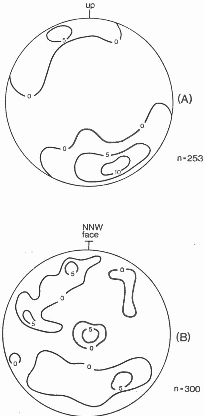
Figure 11. Fabric diagrams for ice sample #1: (A) C-axis distribution of 253 ice crystals from 3 vertical thin sections for planes oriented normal to the thaw face and oblique to the local slope. The sample represents approximately 40% of the total number of crystals visible in the thin sections. (B) C-axis distribution for 300 ice crystals from 3 horizontal thin sections within the sample.
