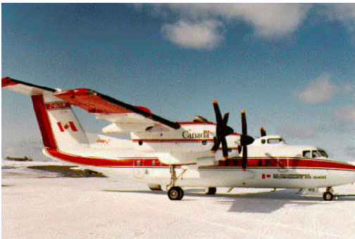
Figure 1: Canadian Ice Service Ice Reconnaissance aircraft C-GCFR equipped with a Side Looking Airborne Radar (SLAR) for both visual and remote sensing observations.
