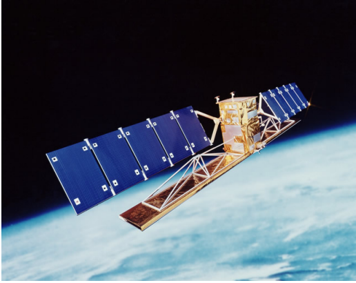
Figure 2: Radarsat Canadian satellite. The main sensor for ice observation is the Synthetic Aperture Radar (SAR).
